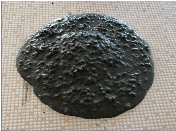
Fig. 8. Slump test of the control mix.
